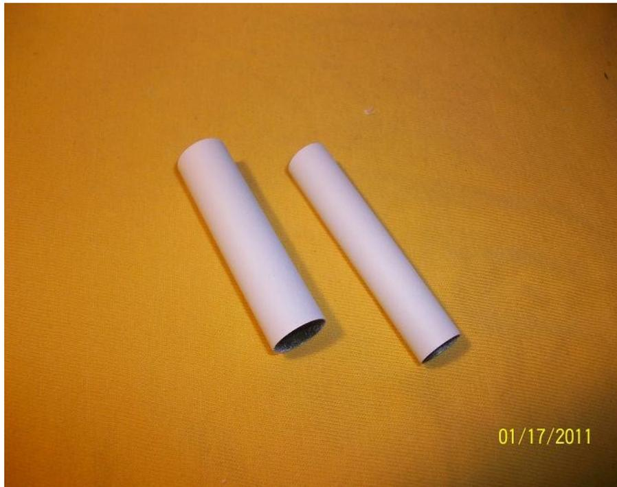
Step 2: You should then cut the skin to length for each tube, leaving a 1/16" excess on both ends. The reason I do this is because the CA sets up fast and I like to have a little excess just in case I mess up.
