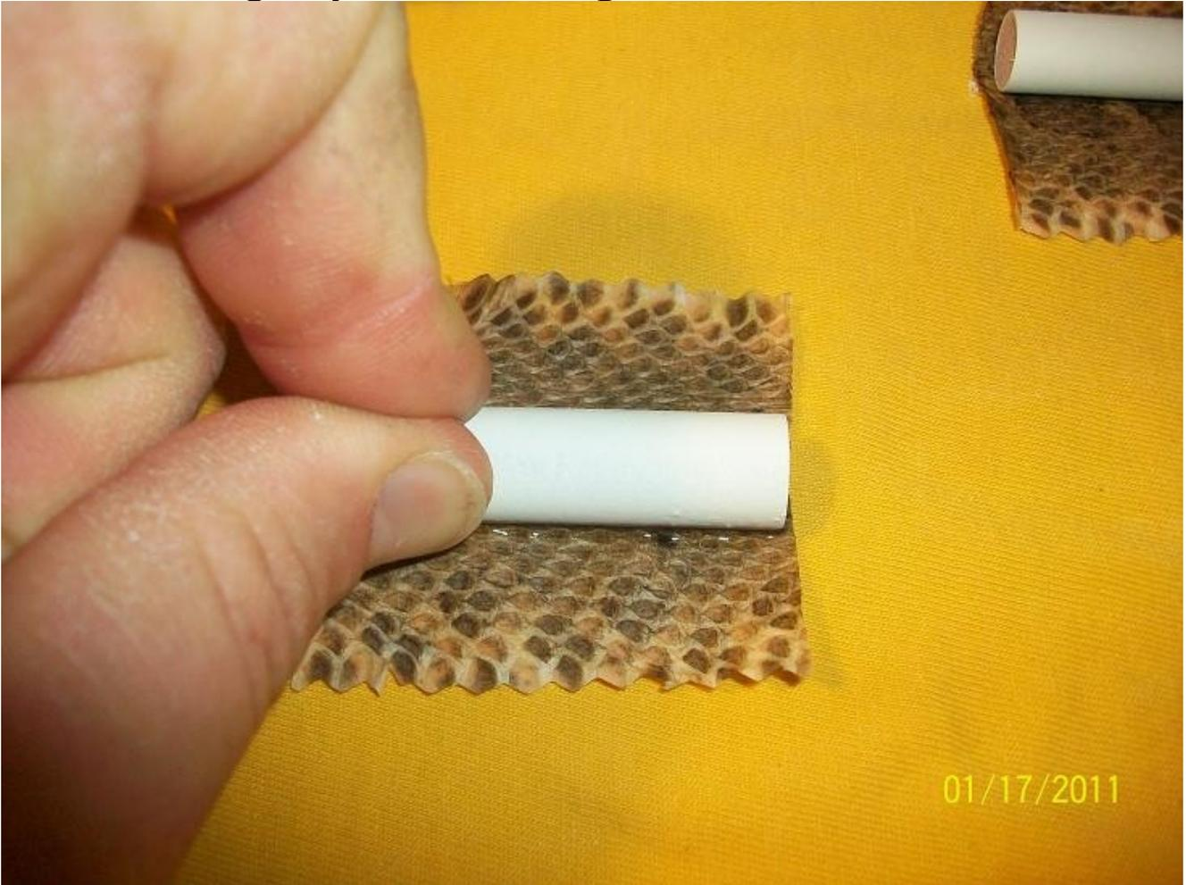
At this point, I apply downward pressure with my fingers making a forward and back rolling motion. This will squeeze the CA to the front and back of the tube and prevent any air pockets from forming. Roll one side all the way over and then the other.
