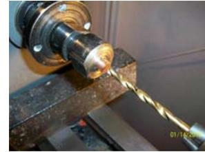
**Use some 3-in-one oil to keep drill bit cool. Again, keep your lathe on the slowest speed during this process. Continue to clear the lead waste as it is drilled by picking it off of the drill bit. I found that the more oil I used, the less locking up of the bit I get. If it does lock up, turn off lathe, and manually twist chuck in reverse(unlock tailstock) and back off the tailstock as you reverse twist the chuck. Drilling complete, leave bullet mounted in chuck.**
