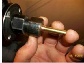
**Step 12: Test fit. Remove bullet from chuck and test fit the Cross ink to**
