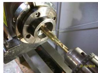
**This last picture is showing how I trim up the drill hole. I use the x-acto knife to do this at a 45 degree angle.**
