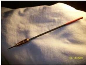
**ensure a proper fit. You want the ink cartridge to stick out through the bullet tip a little farther than what looks normal. If it doesn't, push the bit**
