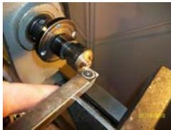
**Step 11: Create the tenon. I use the Easy Rougher for this step. The purpose of this step is to ensure that the brass tube, when inserted into the primer end of the shell, stays**
