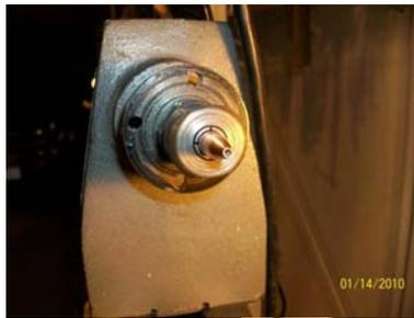
**Step 7: Use a Cross ink refill to test the fit before moving to next step.**
